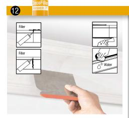
**Use DecoFiller to smooth out all visible joints** I If there are minor irregularities on your coving joints these can be filled with our FL300. You might find it easier to do this 24 hours after the initial installation.
